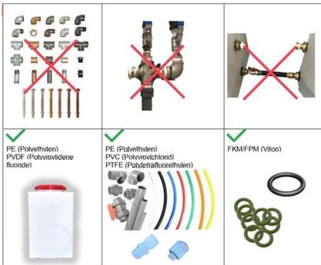
Figure 51 - Neuthox® tank connection requirements
