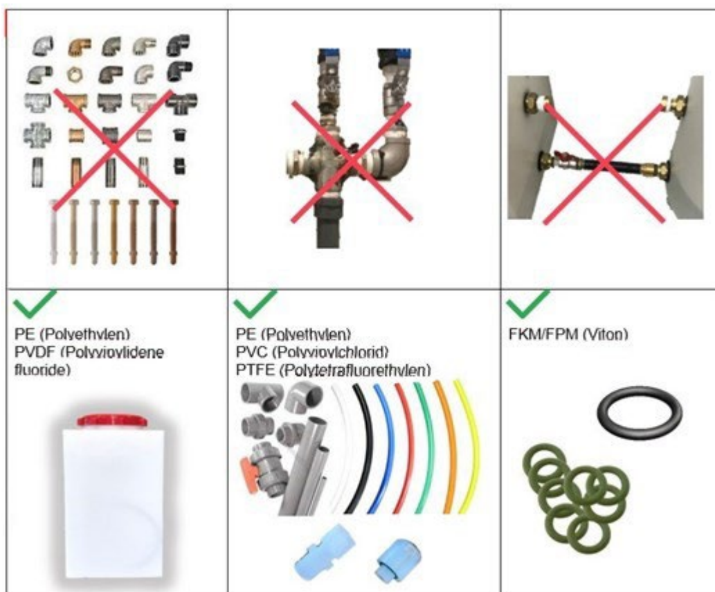
Figure 51 - Neuthox® tank connection requirements
