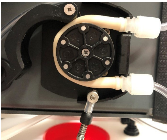
Figure 46 - Pump with hose reinstalled
