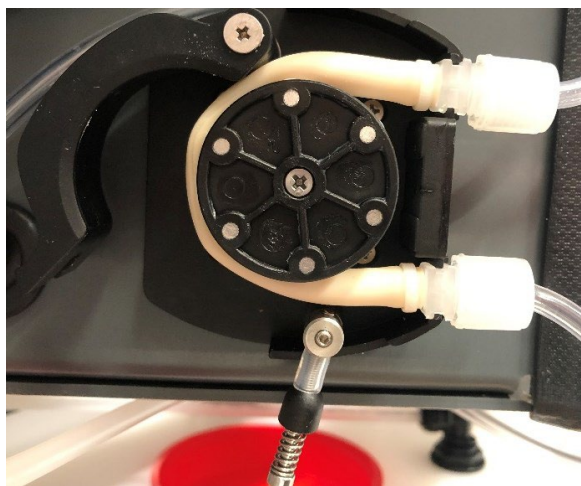
Figure 46 - Pump with hose reinstalled
