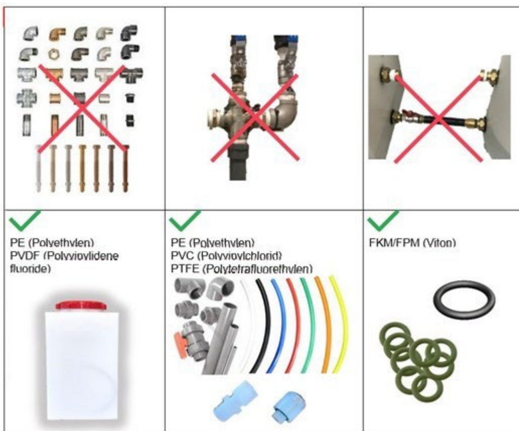
Figure 51 - Neuthox® tank connection requirements
