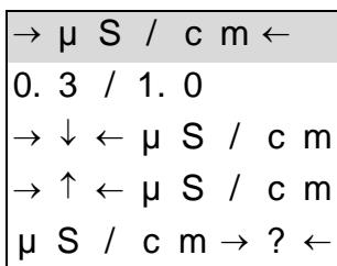
7. Select C-constant according to the chosen conductivity sensor by selecting the highlighted menu option, as shown below. Use arrow keys to choose C-constant, and confirm with “CR” key. The correct sensor (C-constant 0.3 / 1.0) must be used with the relevant range.
