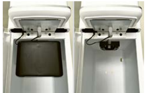
Fig. 5: Interior with wastewater tank in place
