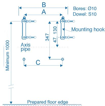
5.4.3. Attach AQA total supply distributor to mounting hooks as shown in diagram and secure with supplied screws.
