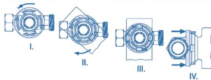
To release the rotation safety, press both clips on the retaining ring together and push upwards with both hands.
