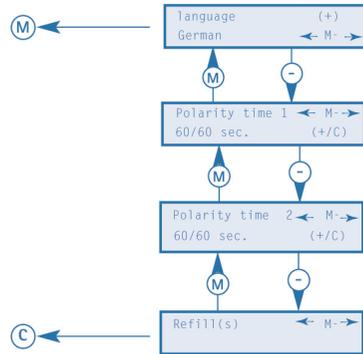
After the refill replacement (usually, all of them), this action must be confirmed to the electronic control system.
