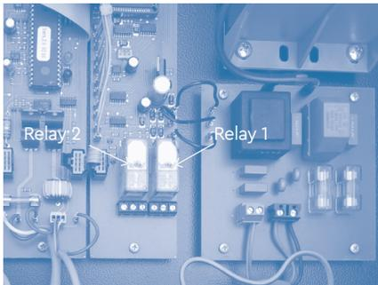
The control relays trigger if a signal is output or if there is a power failure.
