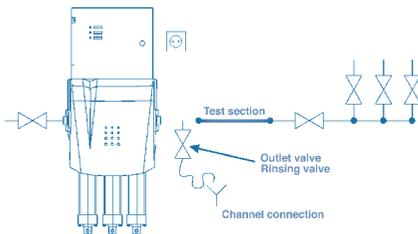
It must be fitted downstream of the AQA total system.
