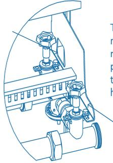
The wall distance can be modified within a certain range by loosening the pre-fixed fixing screws so that the unit is mounted without any stresses.
