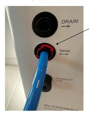
Mount the Female adaptor 8mm (20) to the pressure tanks (14) inlet. Push the 8mm hose (7) into the adaptor (20) and remember to lock it with a locking clip (13).
