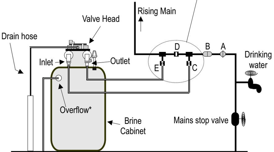
\* The overflow must discharge to a place that is visible outside the building.
