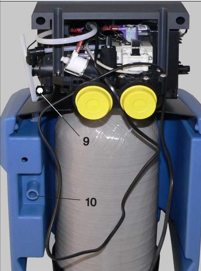
Firmly insert the flushing water hose into the flushing water connection elbow (9).
