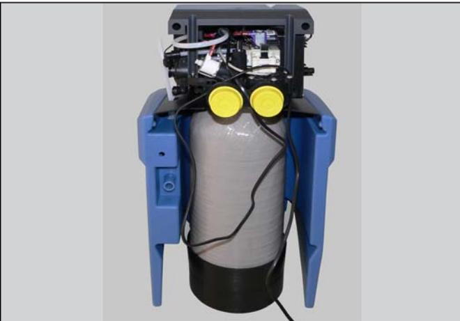
Place and align the softening column with control valve behind the cabinet.
