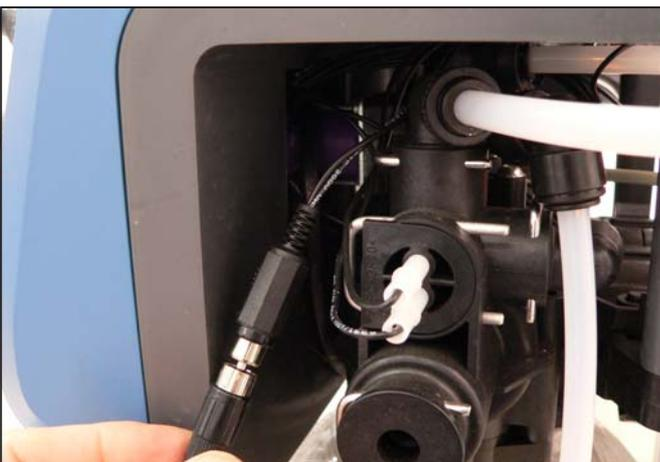
Connect the connection cable with the plugs on the control valve.
