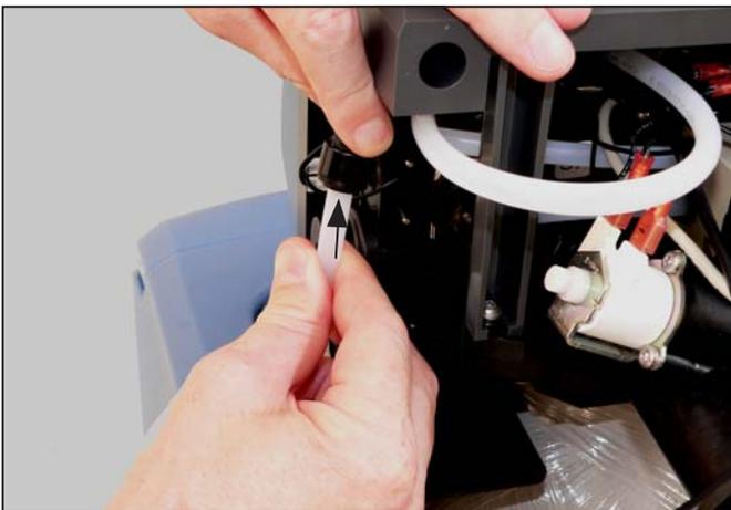
Insert the brine hose into the hose elbow to the limit stop (approx. 15 mm deep).
