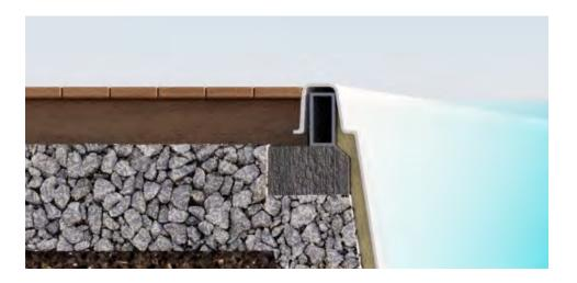
We recommend finishing installation with a 20x25cm concrete ring around the pool perimeter. The ring should be iron rein-forced. Reinforcement bars should be connected to the eyelets of the iron tubes below the pool border.
